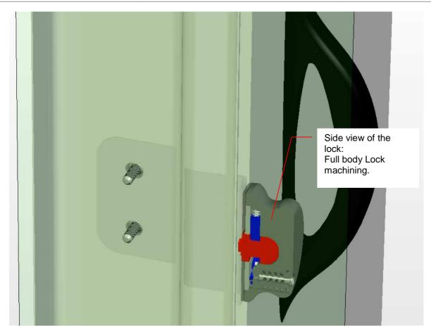
The raw materials (Hardened steel for the body and stainless steel for the cam & peg), the surface treatment (carbonitriding) and the thick of the structure are the natural defense of the lock against drilling or cutting attempts.
