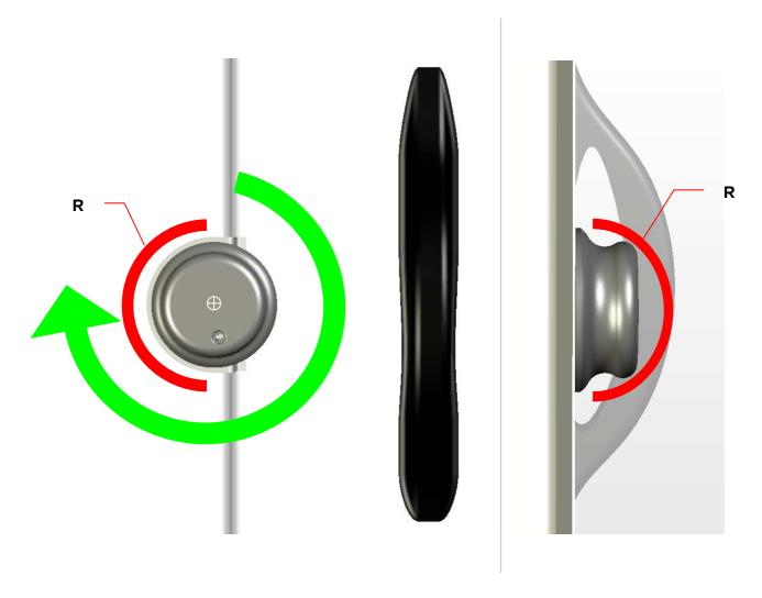
Thanks to its functioning (centering coupling on peg) the lock, once closed, can rotate freely on its axis preventing graspable actions to pull it off.
