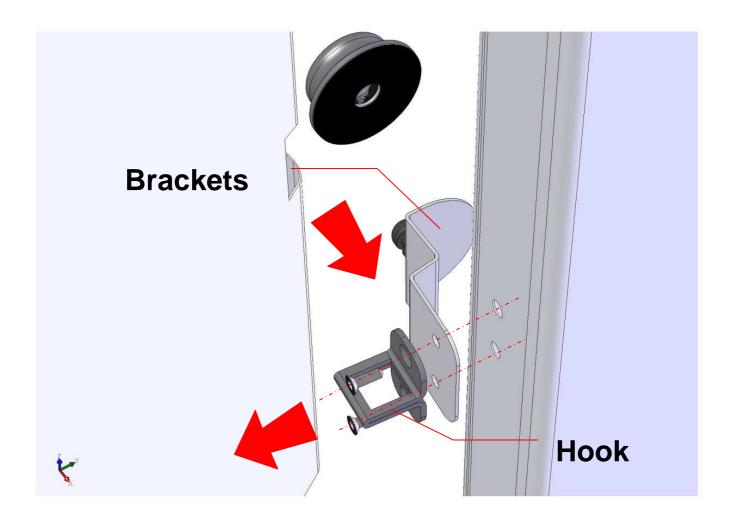
The type of fixation indicated previously, allows the application of the reversible lock. It will be possible to remove the plaque dedicated and tailgate will present the same characteristics as the original, avoiding costly steps to restore the vehicle body.
