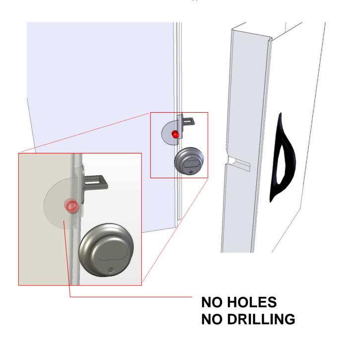
Use the specific shaped plate to fix the lock (which is different from vehicle to vehicle and differs between the rear and the side door). The shaped plate is 3mm thick applied by using the same place of the original lock, over the door sheet metal. This plate is in fact a copy of the profile of the door and therefore perfectly adheres.
