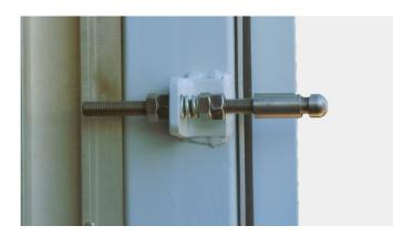
In order to avoid the loss of lock, you can connect it to the frame of the body using a steel cable and eyelet arranged on the lock, taking care not to move with the lock off.
