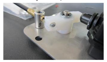
4) Fasten the servo to the inner sheet of the door by using the holes, being careful not to bend the cable of the servo. Too many bends at the elbow causing the retreat of the docking cam, effectively reducing the tightness of the lock.
