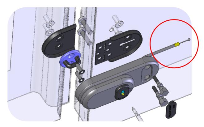
In the event of attempted theft by cutting the sheet metal of the vehicle, GATELOCK VAN has foreseen the use of a sheathed emergency cable to avoid possible hooks and pulls that could cause the doors to open from inside the load compartment.
