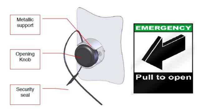
To comply with health & Safety regulations. Allows the driver to open the doors from inside the loading area in case unexpected closing.
