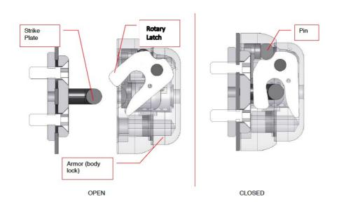
Use the key to open and just slam the door to close the lock and leave the loading area always protected. In case of Deadlocking Operation, the lock remains fitted to the door but it won't close each time the doors are closed. Only if the driver decide it.
